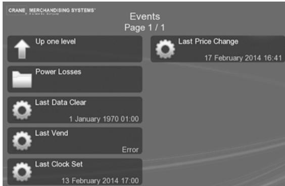
1. **Power Losses** displays a table listing the most recent occasions (10 maximum) when power to the machine was disconnected. Details of the **Date**, **Time** and **Duration** are displayed.
